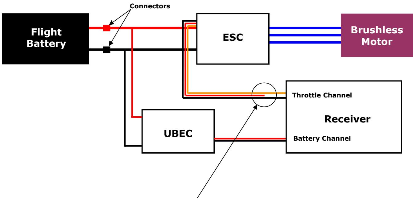
Please note that the red/orange (+ve) wire from the ESC (Electronic Speed Controller) to the receiver is broken. Rather then cut the wire, carefully remove the wire and pin from the plug and tape it back out of the way so that you can re-insert it at a later day if you decide to use the ESC in a different model on a lower voltage.
